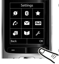
Press right, left, down and up on control key to navigate to the Settings submenu.
