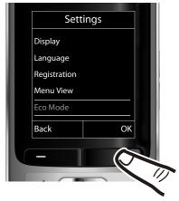
▶ Press down on the control key ↓ until the **Eco Mode** menu option appears on the display.
